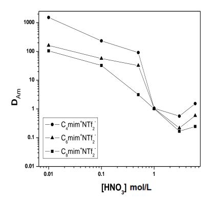
**Figure 7.3.** Distribution constants of Am(III),  $D_{Am}$ , vs. the aqueous nitric acid concentration upon extraction into 1.0 mmol/L T-DGA in  $C_n mim^+$ .NTf<sub>2</sub><sup>-</sup> (n = 4, 6, 8) after 3 h equilibration.
