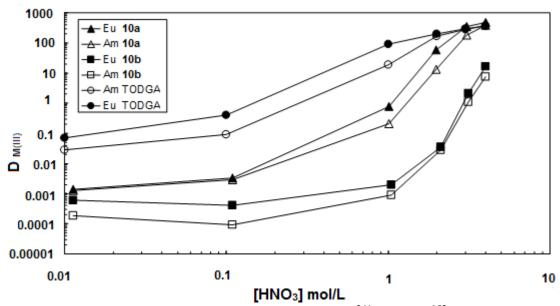
**Figure 3.1**. Nitric acid dependency for the extraction of  $^{241}$ Am and  $^{152}$ Eu by TODGA, **10a** and **10b**. Organic phase: 0.1 mol/L of ligand in TPH. Aqueous phase: variable concentration of nitric acid, tracers:  $^{241}$ Am,  $^{152}$ Eu, mixing time: 15 min; T = 22 °C  $\pm 1$  °C.
