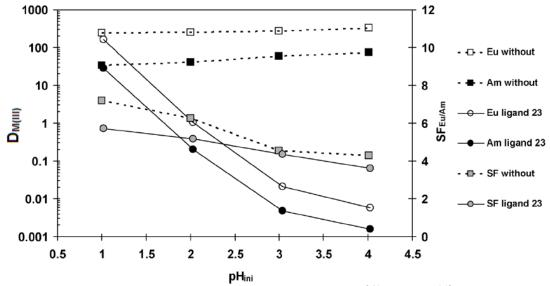
**Figure 4.8**. Initial pH<sub>aq</sub> dependency for the extraction of  $^{241}$ Am and  $^{152}$ Eu. Organic phase: 0.2 mol/L TODGA + 5 vol% 1-octanol in TPH. Aqueous phase: 0.5 mol/L NH<sub>4</sub>NO<sub>3</sub>, variable pH<sub>ini</sub>, 0.1 mol/L ligand **23**, tracers:  $^{241}$ Am,  $^{152}$ Eu, mixing time: 60 min;  $T = 22 \pm 1$  °C.
