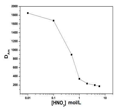
**Figure 7.4.** Distribution constants of Am(III),  $D_{\rm Am}$ , vs. the aqueous nitric acid concentration upon extraction into  $7\times10^{-4}$  mol/L C4DGA in C<sub>8</sub>mim<sup>+</sup>.PF<sub>6</sub>.
