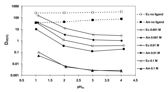
**Figure 4.5**. Initial pH<sub>aq</sub> and ligand **17** concentration dependency for the extraction of  $^{241}$ Am and  $^{152}$ Eu. Organic phase: 0.2 mol/L TODGA + 5 vol% 1-octanol in TPH. Aqueous phase: 0.5 mol/L NH<sub>4</sub>NO<sub>3</sub>, variable pH<sub>ini</sub>, variable concentration of ligand (**17**), tracers:  $^{241}$ Am,  $^{152}$ Eu, mixing time: 60 min;  $T = 22 \pm 1$  °C.
