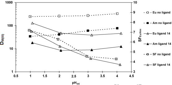
**Figure 4.4**. Initial pH<sub>aq</sub> dependency for the extraction of  $^{241}$ Am and  $^{152}$ Eu. Organic phase: 0.2 mol/L TODGA + 5 vol% 1-octanol in TPH. Aqueous phase: 0.5 mol/L NH<sub>4</sub>NO<sub>3</sub>, variable pH<sub>ini</sub>, ligand **14** <0.03 mol/L, tracers:  $^{241}$ Am,  $^{152}$ Eu, mixing time: 60 min;  $T = 22 \pm 1$ °C.
