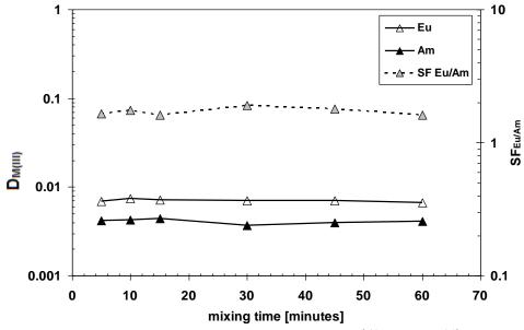
**Figure 4.6**. Mixing time dependency for the extraction of  $^{241}$ Am and  $^{152}$ Eu. Organic phase: 0.2 mol/L TODGA + 5 vol% 1-octanol in TPH. Aqueous phase: 0.5 mol/L NH<sub>4</sub>NO<sub>3</sub>, 0.1 mol/L ligand **17**, pH<sub>ini</sub> = 4, variable mixing time, tracers:  $^{241}$ Am,  $^{152}$ Eu;  $T = 22 \pm 1$  °C.
