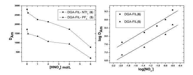
**Figure 8.2** left: a) Relative extraction profiles of Am(III) in DGA-FILs **5** and **6** as a function of aqueous phase acid concentration. right: b) Dependence of Am(III) extraction on aqueous phase nitrate ion concentration; Aqueous phase: 0.01 mol/L HNO<sub>3</sub> + varying amounts of NaNO<sub>3</sub>.
