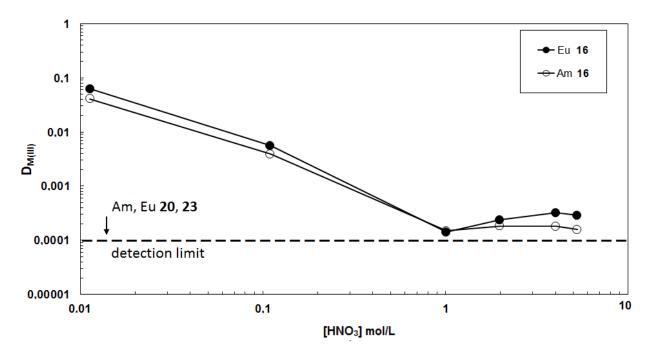
**Figure 6.4**. Nitric acid dependency for the extraction of  $^{241}$ Am and  $^{152}$ Eu by ligand **16**. Organic phase: 0.1 mol/L **16** in TPH. Aqueous phase: variable concentration of nitric acid, tracers:  $^{241}$ Am and  $^{152}$ Eu, mixing time: 60 min;  $T = 22 \pm 1$  °C.
