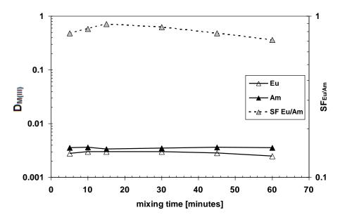
**Figure 4.2.** Mixing time dependency for the extraction of  $^{241}$ Am and  $^{152}$ Eu. Organic phase: 0.2 mol/L TODGA + 5 vol% 1-octanol in TPH. Aqueous phase: 0.5 mol/L NH<sub>4</sub>NO<sub>3</sub>, 0.1 mol/L ligand (2), pH<sub>ini</sub> = 3, variable mixing time, tracers:  $^{241}$ Am,  $^{152}$ Eu;  $T = 22 \pm 1$  °C.
