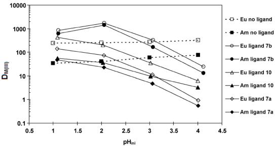
**Figure 4.3**. Initial pH<sub>aq</sub> dependency for the extraction of  $^{241}$ Am and  $^{152}$ Eu. Organic phase: 0.2 mol/L TODGA + 5 vol% 1-octanol in TPH. Aqueous phase: 0.5 mol/L NH<sub>4</sub>NO<sub>3</sub>, variable pH<sub>ini</sub>, 0.1 mol/L ligand **7a**, **7b** (0.01 mol/L ligand **10**), tracers:  $^{241}$ Am,  $^{152}$ Eu, mixing time: 60 min;  $T = 22 \pm 1$  °C.
