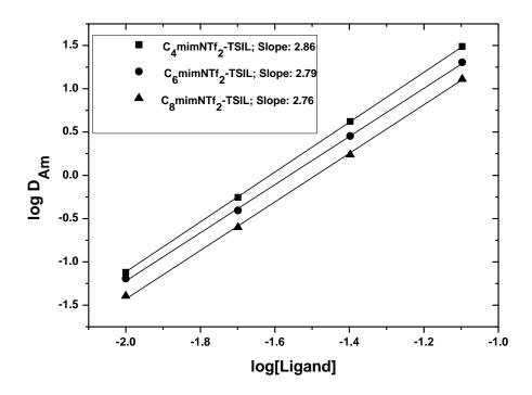
**Figure 8.5.** Effect of variation of CMPO-FIL (**10**) concentration versus Am(III) distribution. Aqueous phase: 3 mol/L HNO<sub>3</sub>. Organic phase: CMPO-FIL in C<sub>n</sub>min.NTf<sub>2</sub>.
