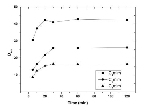
**Figure 8.6.**  $D_{Am}$  values as a function of time for CMPO-FIL (10) in [C<sub>n</sub>mim][NTf<sub>2</sub>] at 3 mol/L HNO<sub>3</sub>.
