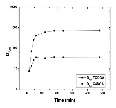
**Figure 7.2.** Distribution constants of Am(III),  $D_{Am}$ , vs. time using 1.0 mmol/L C4DGA and 10 mmol/L TODGA in  $C_8mim^+$ .PF<sub>6</sub> and 3 mol/L HNO<sub>3</sub> feed.
