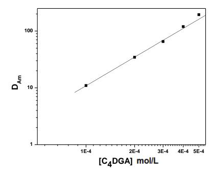
**Figure 7.6.** Distribution ratio of Am(III),  $D_{Am}$ , vs. the C4DGA concentration upon extraction from 3 mol/L HNO<sub>3</sub> feed into  $C_8$ mim<sup>+</sup>.PF<sub>6</sub>.
