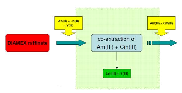
Figure 2.2. Schematic view of the SANEX process.
