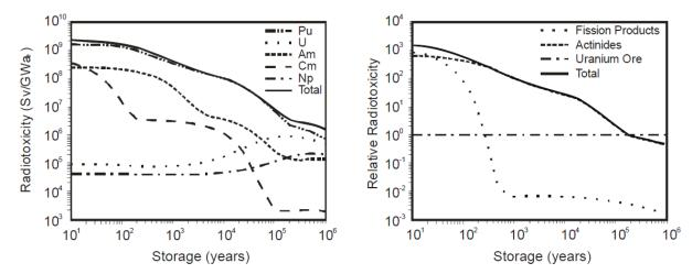
**Figure 1.1.** Left: The radiotoxicity per element of the actinides in spent  $U(VI)O_2$  fuel. (GWae is a measure of electricity produced and 1 GWae equals about two times the annual production of the Borssele nuclear power plant). Right: The radiotoxicity of the actinides and fission products in spent fuel relative to the uranium ore needed to manufacture the fuel. The storage time needed to reach a radiotoxicity level of uranium ore is about 200,000 years.<sup>5</sup>
