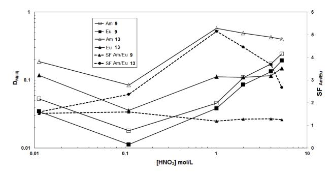
**Figure 6.3**. Nitric acid dependency for the extraction of  $^{241}$ Am and  $^{152}$ Eu by ligands **9** and **13**. Organic phase: 0.1 mol/L ligand in TPH. Aqueous phase: variable concentration of nitric acid, tracers:  $^{241}$ Am and  $^{152}$ Eu, mixing time: 60 min;  $T = 22 \pm 1$  °C.
