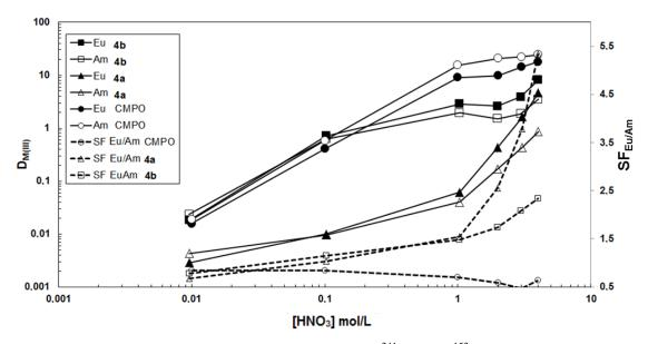
**Figure 6.1**. Nitric acid dependency for the extraction of <sup>241</sup>Am and <sup>152</sup>Eu by ligands **4a,b** and comparison with CMPO/TBP.
