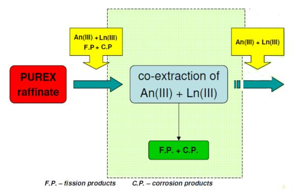
Figure 2.1. Co-extraction of An(III) and Ln(III) from the PUREX raffinate.
