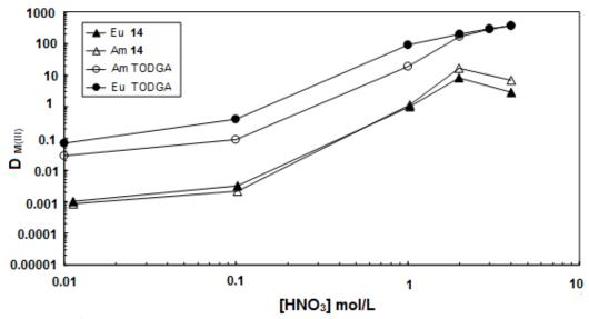
**Figure 3.3**. Nitric acid dependency for the extraction of  $^{241}$ Am and  $^{152}$ Eu by TODGA and **14**. Organic phase: 0.1 mol/L of TODGA or 0.08 mol/L of **14** in TPH. Aqueous phase: variable concentration of nitric acid, tracers:  $^{241}$ Am,  $^{152}$ Eu, mixing time: 15 min TODGA (60 min ligand **14**);  $T = 22 \, ^{\circ}$ C  $\pm 1 \, ^{\circ}$ C.
