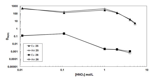
**Figure 6.5**. Nitric acid dependency for the extraction of <sup>241</sup>Am and <sup>152</sup>Eu by ligands **25** and **26**. Organic phase: 0.1 mol/L **26** in TPH or 0.09 mol/L **25** + 0.003 mol/L 1-octanol in TPH (due to a lower solubility of **25** in pure TPH).
