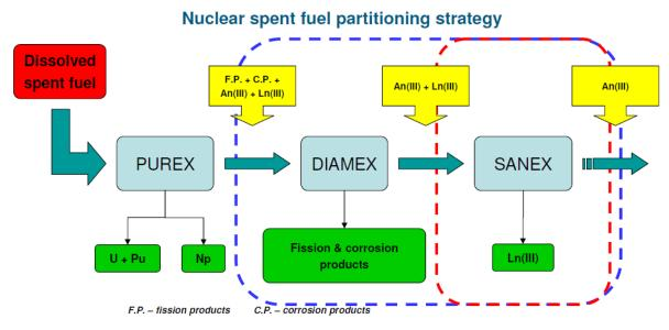
**Figure 1.2**. Schematic view of the partitioning process of actinides (courtesy of Dr. G. Modolo).
