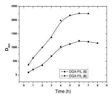
**Figure 8.1**.  $D_{Am}$  values as a function of time for DGA-FILs **5** and **6** at 3 mol/L HNO<sub>3</sub>.
