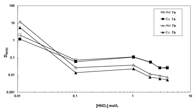
**Figure 6.2**. Nitric acid dependency for the extraction of  $^{241}$ Am and  $^{152}$ Eu by ligands **7a,b**. Organic phase: 0.1 mol/L ligand in TPH. Aqueous phase: variable concentration of nitric acid, tracers:  $^{241}$ Am and  $^{152}$ Eu, mixing time: 60 min;  $T = 22 \pm 1$  °C.
