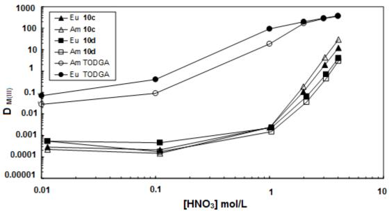
**Figure 3.2**. Nitric acid dependency for the extraction of  $^{241}$ Am and  $^{152}$ Eu by TODGA, **10c** and **10d**. Organic phase: 0.1 mol/L of ligand in TPH. Aqueous phase: variable concentration of nitric acid, tracers:  $^{241}$ Am,  $^{152}$ Eu, mixing time: 15 min; T = 22 °C ± 1 °C.
