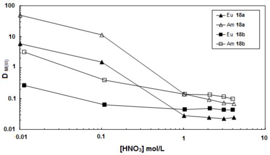
**Figure 3.4**. Nitric acid dependency for the extraction of  $^{241}$ Am and  $^{152}$ Eu by **18a** and **18b**. Organic phase: 0.1 mol/L of the ligand in TPH. Aqueous phase: variable concentration of nitric acid, tracers:  $^{241}$ Am,  $^{152}$ Eu, mixing time: 15 min; T = 22 °C ± 1 °C.
