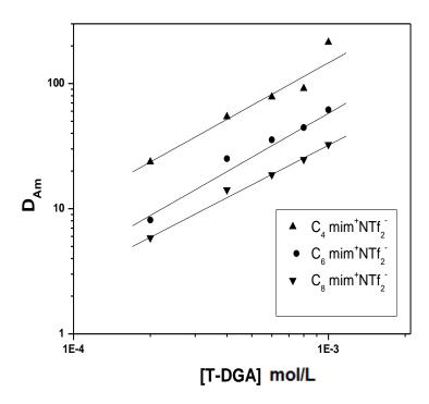
**Figure 7.5.** Distribution ratio of Am(III),  $D_{Am}$ , vs. the T-DGA concentration upon extraction from 0.5 mol/L HNO<sub>3</sub> feed into  $C_n mim^+$ .NTf<sub>2</sub><sup>-</sup> (n = 4, 6, 8).
