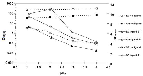
**Figure 4.7**. Initial pH<sub>aq</sub> dependency for the extraction of  $^{241}$ Am and  $^{152}$ Eu. Organic phase: 0.2 mol/L TODGA + 5 vol% 1-octanol in TPH. Aqueous phase: 0.5 mol/L NH<sub>4</sub>NO<sub>3</sub>, variable pH<sub>ini</sub>, 0.07 mol/L ligand **21**, tracers:  $^{241}$ Am,  $^{152}$ Eu, mixing time: 60 min;  $T = 22 \pm 1$  °C.
