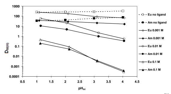
**Figure 4.1**. Initial pH<sub>aq</sub> and ligand (2) concentration dependency for the extraction of  $^{241}$ Am and  $^{152}$ Eu. Organic phase: 0.2 mol/L TODGA + 5 vol% 1-octanol in TPH. Aqueous phase: 0.5 mol/L NH<sub>4</sub>NO<sub>3</sub>, variable pH<sub>ini</sub>, variable concentrations of ligand **2**, tracers:  $^{241}$ Am,  $^{152}$ Eu, mixing time: 60 min;  $T = 22 \pm 1$  °C.
