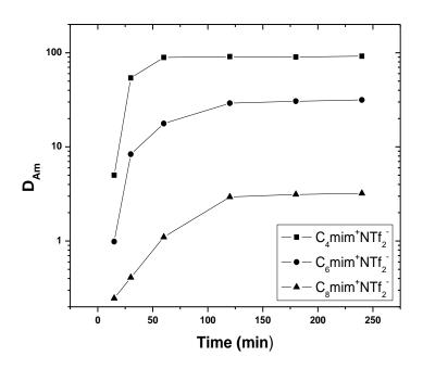
**Figure 7.1.** Distribution constants of Am(III),  $D_{Am}$ , vs. time using 1.0 mmol/L T-DGA in  $C_n mim^+.NTf_2^-$  (n = 4, 6, 8) and a 0.5 mol/L HNO<sub>3</sub> feed.
