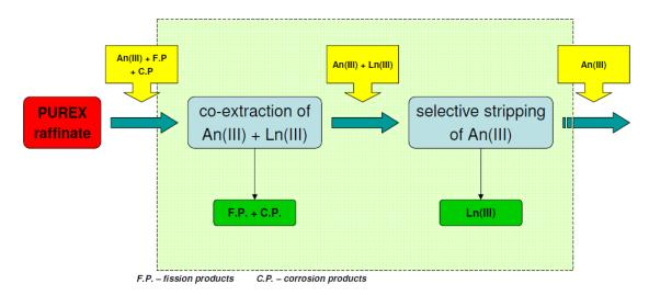
Figure 2.3. Schematic overview of the innovative SANEX process.
